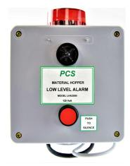
PCS Company's Low Level Material Hopper Alarm eliminates machine shutdowns caused by empty hoppers. The alarm uses a proximity sensor to monitor the material level in the machine hopper. If the material level drops below the sensor, a loud alarm sounds and a flashing red light alerts plant personnel. The low level alarm can be used in various processes such as injection molding, blow molding and extrusion. Simple installation requiring 110v and a 1-1/4" hole in the hopper.
